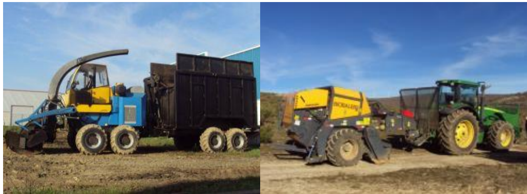
Figure 12: Example of novel implements utilised in the ENERBIOSCRUB project for collecting shrub biomass. Left: Papamato shredder; right: Anderson's Biobaler (pictures available at http://enerbioscrub.ciemat.es/ ).
