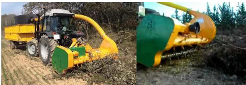
Figure 11: Example of shredder able to obtain woodchips from longitudinal piles (Pictures: www.serrat.es ).
