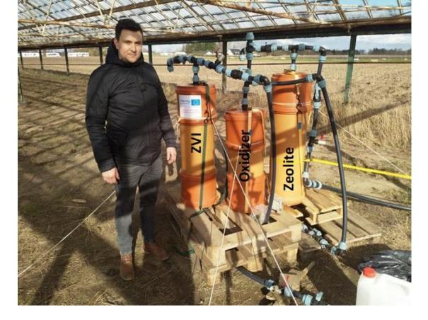
University of Copenhagen is testing a so-called Zero Valent Iron (ZVI) filter for nitrate filtration at its Taastrup Campus. Through this filter, the nitrate in drainage water is being reduced to ammonium by metallic iron (ZVI), and the ammonium produced is being retained on a zeolite cation exchanger. The new idea is to recycle nitrogen.
